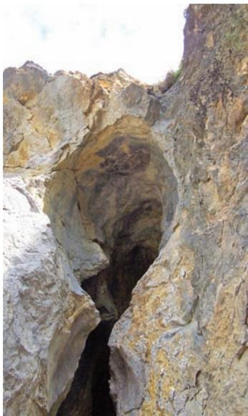
Fig. 5. Roșia Montană: work opened by fire-setting at the "Găuri" site.
