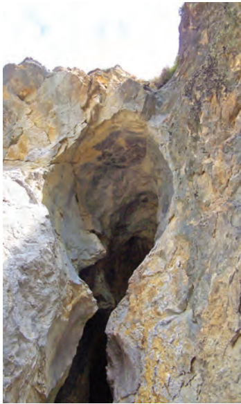
Fig. 5. Roşia Montană: work opened by fire-setting at the "Găuri" site.
