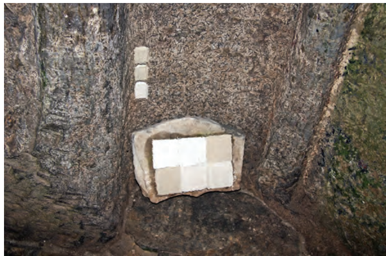
Fig. 5. Samples of different compositions of mortars destined to the consolidation intervention at the painting support have been tested by CEPROCIM S.A. Not only was the compatibility with original materials examined, but the behaviour of new mortars in severe microclimate conditions, too.
