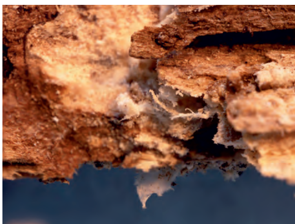
Fig. 12. Wood sample colonized in-depth by consecutive masses of mycelium ( Phellinus sp.; x = 80).
