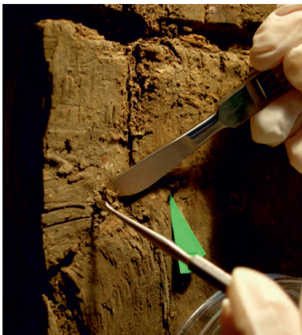
Fig. 7. On sample harvesting for microbiological analysis, it was found that the wood is friable.
