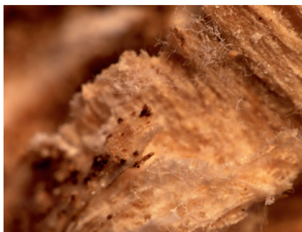
Fig. 13. Wood sample colonized by aerial and submerged mycelium ( Antrodia sinuosa ; x = 80).
