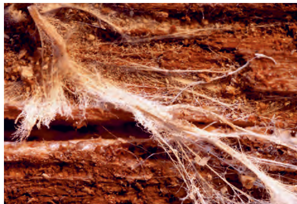
Fig. 17. Strands of Antrodia sinuosa identified at the surface of the wood sample (x = 80).
