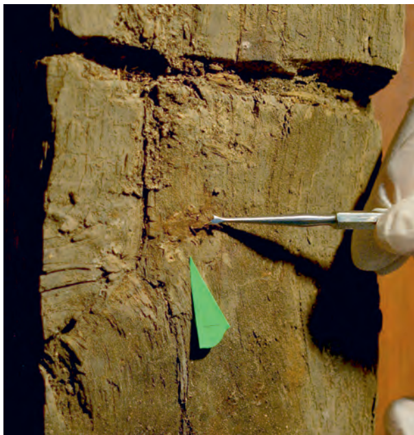
Fig. 4. Wood sample covered by brown thick mycelium.
