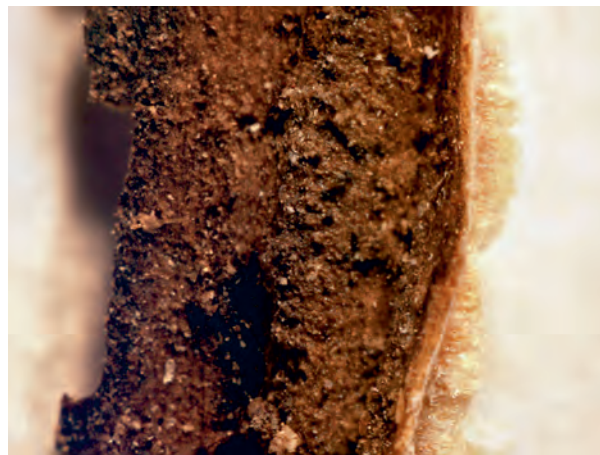
Fig. 5. The top surface of the sample confirms, by optical microscopy, the existence of thick, brown mycelium and deposits ( Phellinus sp.; magnification \times 80 ).
