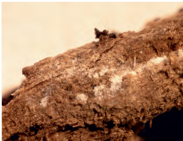
Fig. 10. Brown coloured wood sample colonized on the surface by white and viable mycelium of Antrodia sinuosa (x = 40).
