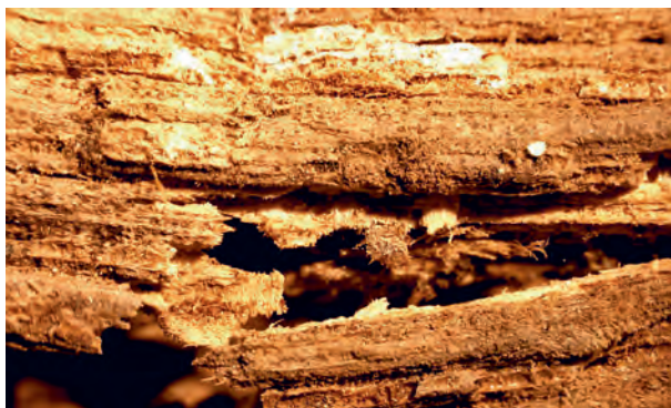
Fig. 8. Deep into the wood consecutive layers of mycelium developed by Antrrodia sinuosa ( x = 80 ) were revealed.
