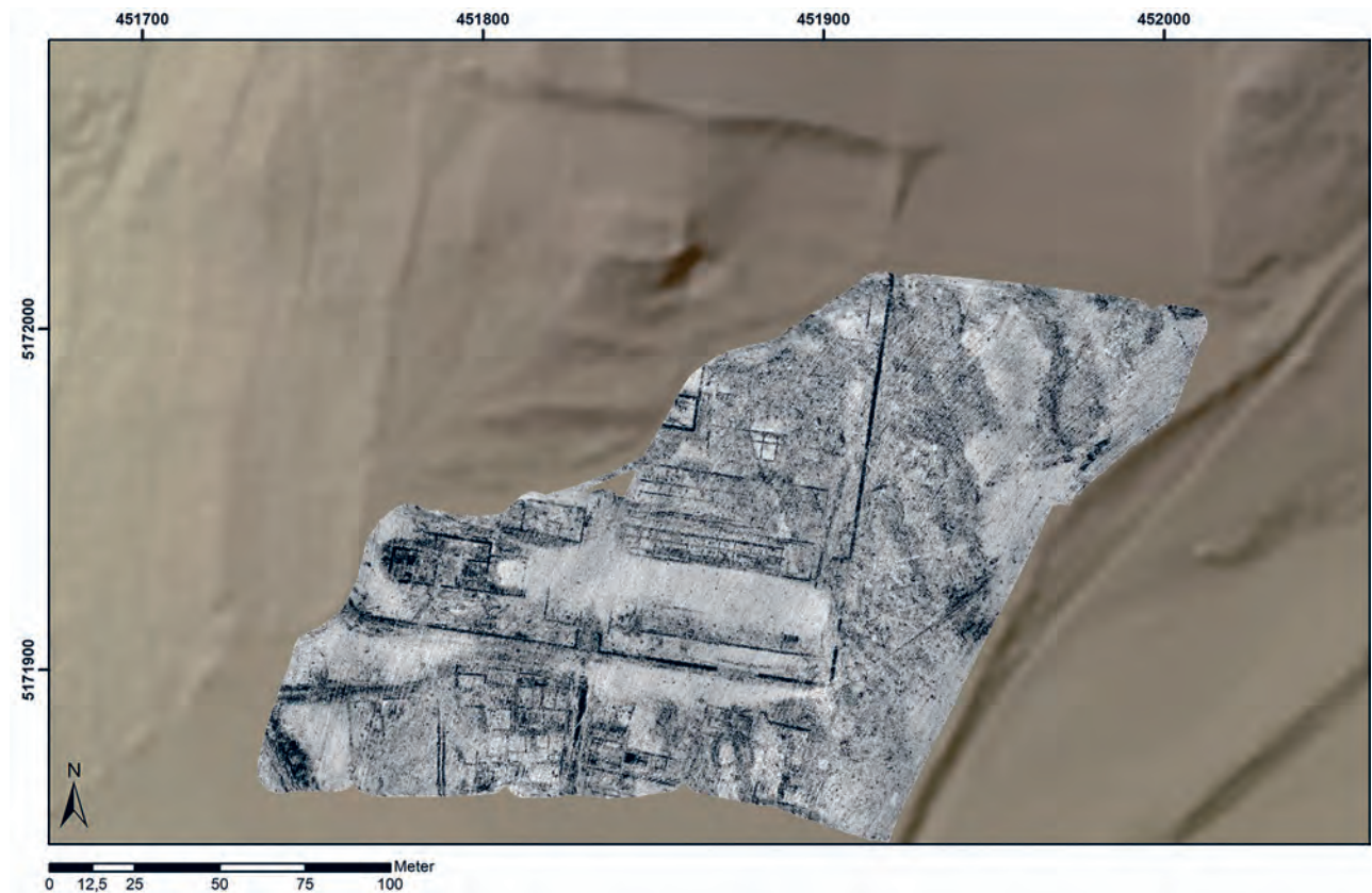
Fig. 4. Ground-penetrating radar measurements taken during 2013. The accumulated depth slices measure between 60 and 90 centimetres below surface level (© 2013 Ludwig-Boltzmann-Institut für Archäologische Prospektion und Virtuelle Archäologie (LBI ArchPro)).
